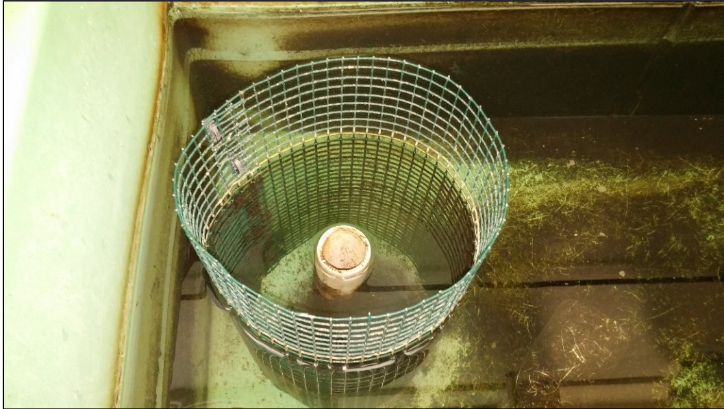
Figure 4. Overflow pipe and PVC-coated hardware cloth cylinder. The overflow pipe limits water depth to a maximum of 13 inches. During water exchanges, the pipe is removed manually from the drain opening to allow 3 to 4 inches of water to drain from the tub. The hardware cloth cylinder allows particulate debris and animal wastes to accumulate at the base of the overflow pipe for subsequent flushing from the tank during water exchanges. In Figure 3 above, note the presence of weights positioned atop the cylinder. The pressure applied to the cylinder by these weights prevents frogs from passing under the cylinder and near the overflow pipe.
