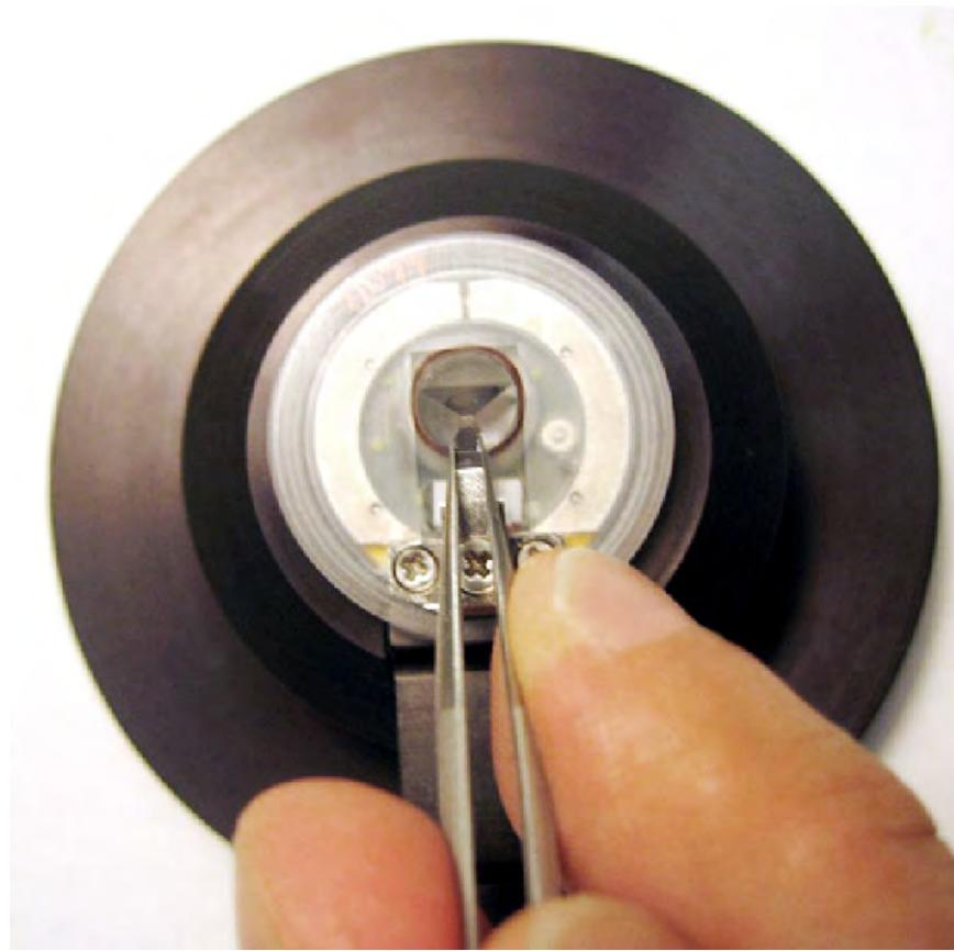
*Figure 5.13 Inserting a Cantilever*
