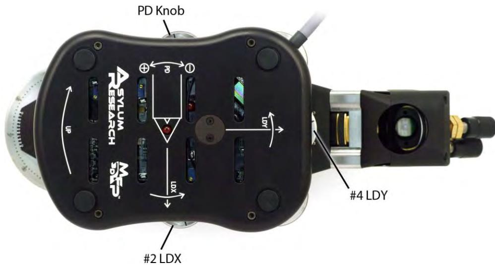
Figure 5.15 Optical Detector Adjustments (PD, LDY and LDX)
