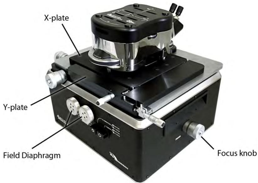
Figure 5.21 Bottom View Camera X and Y Position
