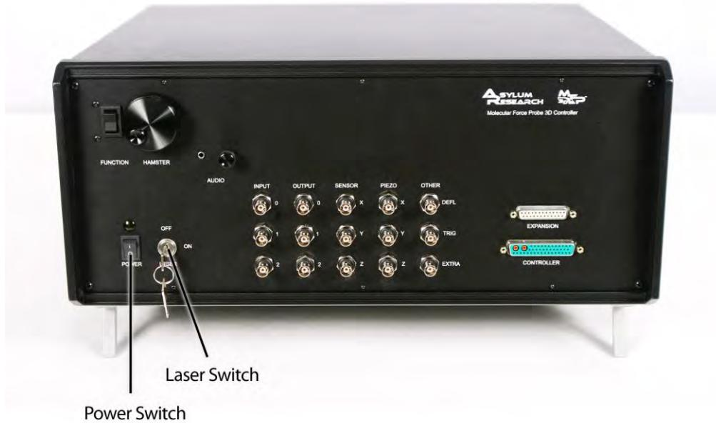
*Figure 4.13 Controller Power*
