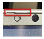
Some newer laptops have a built-in privacy shutter that covers the lens above the laptop screen. This slider door can be difficult to see and many are unaware of its existence. If the slider door inadvertently gets closed, it can seem as though the camera is not working as the video on the screen will appear dark even if video is turned on. This can be especially problematic during video calls.
