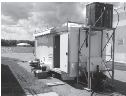
The Mobile Exposure Laboratory Trailer (MELT), a complete, self-contained laboratory facility belonging to the SCSU Aquatic Toxicology Laboratory setup for exposure experiments at a wastewater treatment plant facility in Minnesota.
