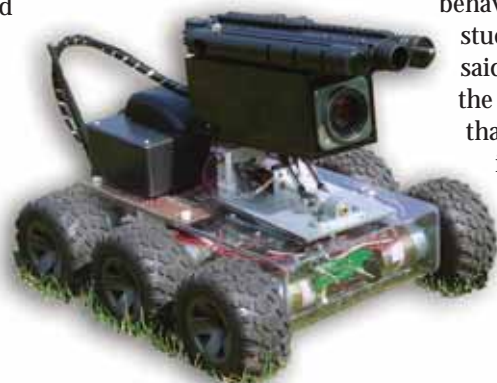
The UGVs’ mission in 2005 was to mark (shoot accurately at) targets with paint balls.
