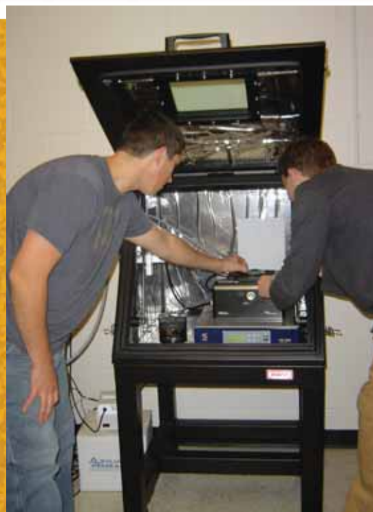
Cody Gebhardt, left, and Bob Janisch mount a crystal sample for scanning with the SPM.
