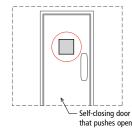
not on a hold-open device. For example, restroom doors that push open into the restroom, and the door automatically closes, may have the tactile identification sign installed on the door. (Illustration 2)
